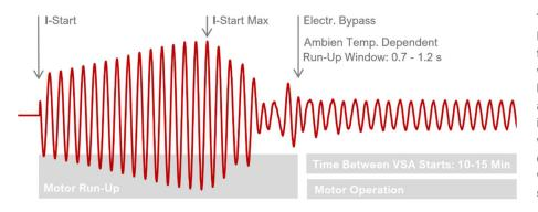
The arrangement of switched NTC thermistors is in its function a full wave softstarter, without any harmonics caused by phase angle control. This allows the softstarter to be integrated into the existing wiring of any on/off climate control compressor setup without additional components such as filters.
