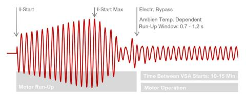
The arrangement of switched NTC thermistors is in its function a full wave softstarter, without any harmonics caused by phase angle control. This allows the softstarter to be integrated into the existing wiring of any on/off climate control compressor setup without additional components such as filters.
